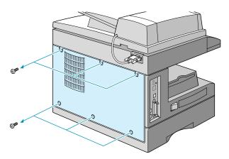
4 Pull the control board cover slightly towards you and slide it to the left. Remove the cover from the machine.
